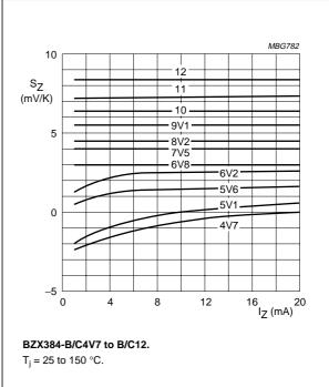
Fig.5 Temperature coefficient as a function of working current; typical values.
